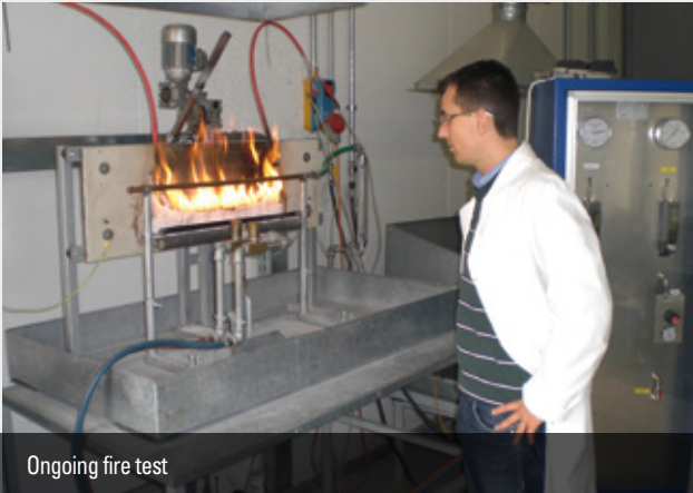
Flame and mechanical shock BS 50200
